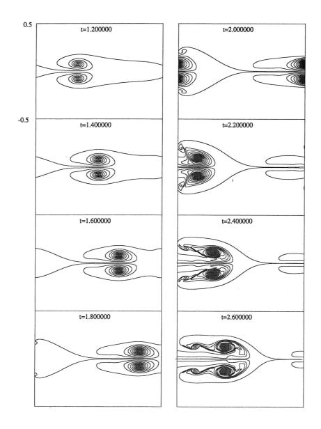
Figure 2: Long time evolution of two vortex sheets. The initial parameters are H=0.2,  $\alpha=1.0$ ,and  $(\sigma_1,\sigma_2)=(1,-1)$ .
