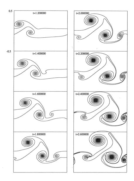
Figure 1: Long time evolution of two vortex sheets. The initial parameters are H=0.2,  $\alpha=0.0$ ,and  $(\sigma_1,\sigma_2)=(1,-1)$ .
