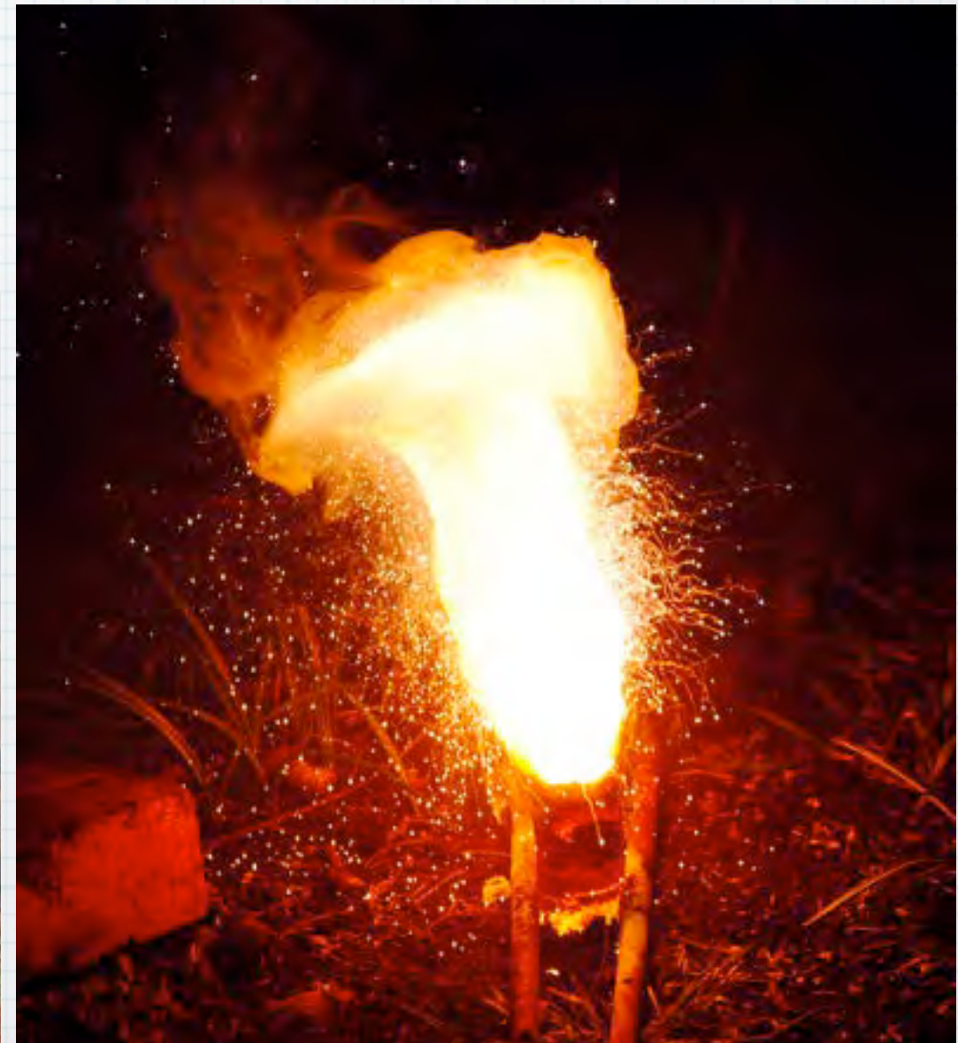
A thermite reaction using iron(III) by Nikthestonea
